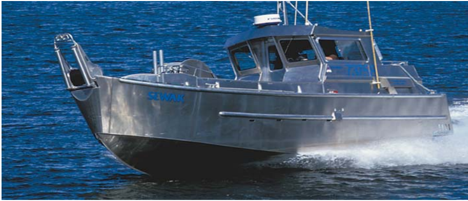
When time is money, speed is important, and gillnetters like this aluminum bowpicker operate at 20 knots or so even in dense fog. Making sure the radar is performing at peak efficiency is critical.
